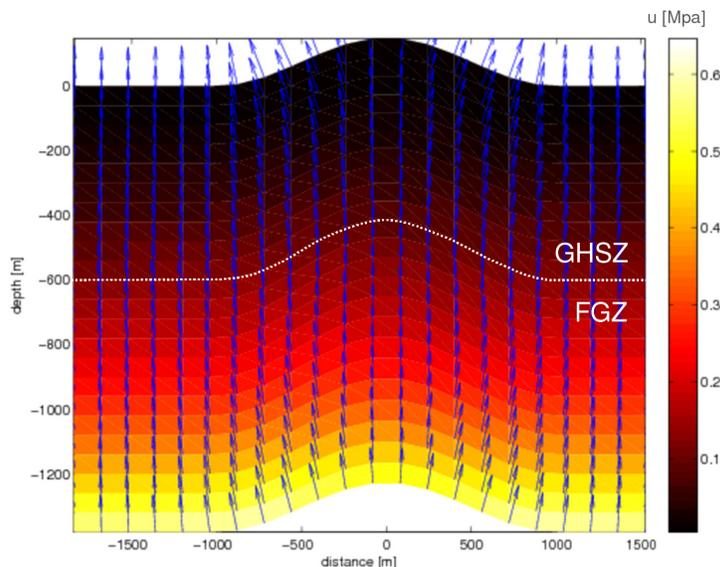
Figure 18: Overpressure and fluid flow induced in a ridge structure by continuous sedimentation. [J. Hauschildt]
