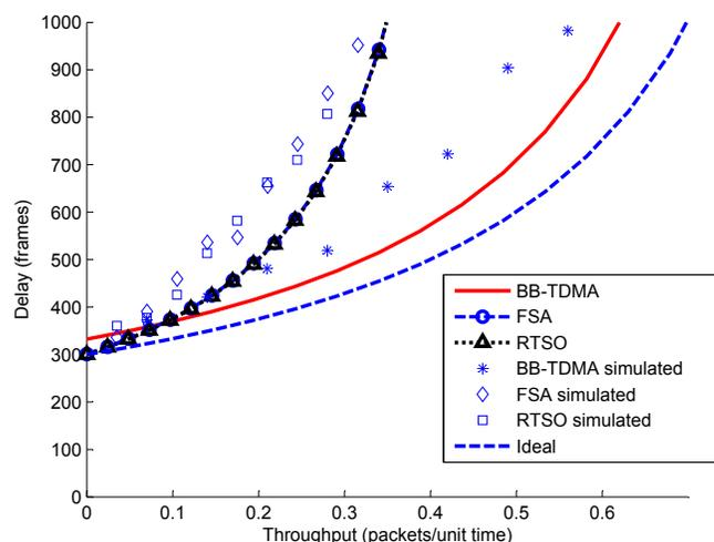
Figure 6: Throughput-delay results of new medium access control (MAC) protocol for hybrid cellular and *ad hoc* 4th generation wireless networks. [H. Haas et al.]
