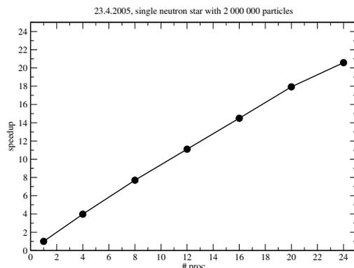
Figure 14: Speedup of the smoothed particle hydrodynamics code developed for neutron star collisions. [S. Rosswog]
