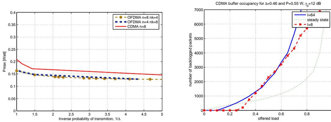
Figure 36: Power control and link scheduling project of the CWC group. Left: Pareto optimal curves for CDMA and OFDMA, obtained for the same  $N_c$  number of subcarrier per system. Right: Mean buffer occupancy for CDMA uplink. [H. Haas]
