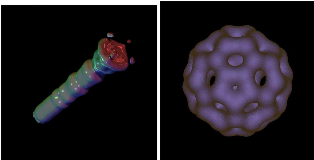
Figure 6: Left: Point-based ray tracing of isosurface directly extracted from scattered volume data. The scattered data set is a uniform random sampling of simulation data of fuel injection into a combustion chamber. Right: Exact dual isosurfacing using ray intersection applied to simulation of electron density inside a C-60 Buckminsterfullerene. [L. Linsen]
