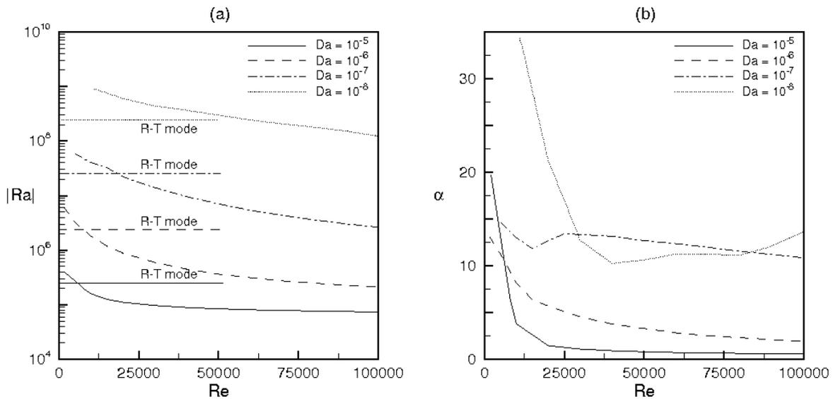
Figure 39: Dependence of the critical Rayleigh number (a) and wave number (b) on  $Re$  for different Darcy numbers at  $Pr = 7$ . [A. Khalili]
