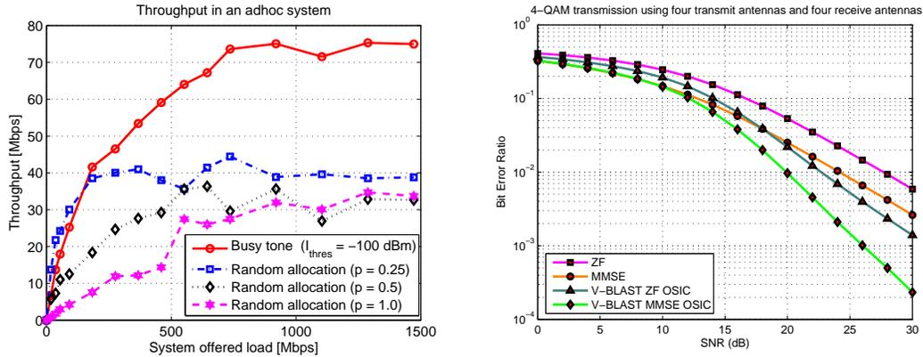
Figure 37: Projects of the CWC group. Left: Interference avoidance using the busy tone concept. Comparison of throughput in different channel allocation scheme. Right: MIMO systems. BER vs. SNR for 4-QAM spatial multiplexing transmission using four transmit and receive antennas. [H. Haas]
