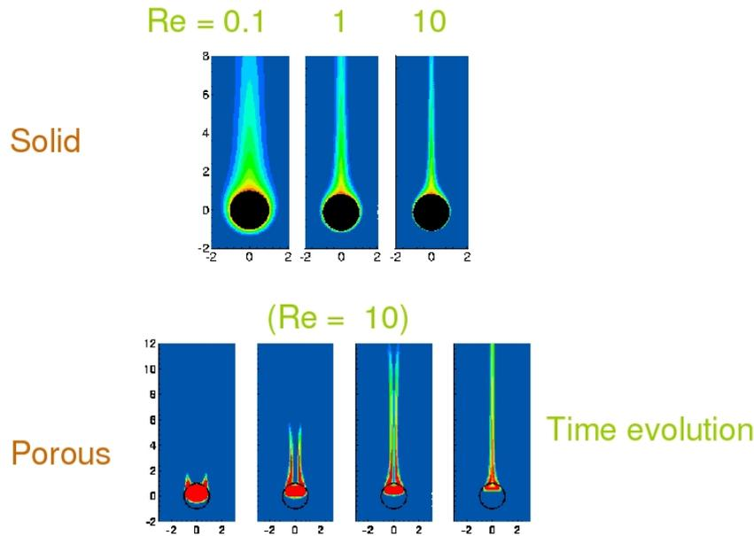
Figure 38: Comparison of fluid flow around a solid aggregate vs the same through and around a porous one. [A. Khalili]
