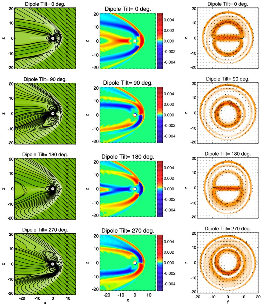
Figure 31: Diurnal variations in an equatorial dipolar paleomagnetosphere. Figures taken from Zieger et al. (2004). Left: Magnetic field lines and pressure distribution. Center: Currents flowing across the equatorial plane. Right: Tail current systems. [J. Vogt and B. Zieger]
