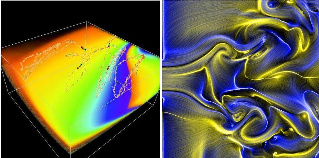
Figure 7: Left: Visualization of streaming temperature data in Monterey Bay scattered over time and space. A direct volume rendering of a three-dimensional time-orthogonal hyperplane after reconstruction over a  $128 \times 128 \times 64 \times 1800$  grid (using natural neighbor interpolation) is shown. Right: Structure-accentuating dense flow visualization applied to 2D simulation of a swirling jet. [L. Linsen]
