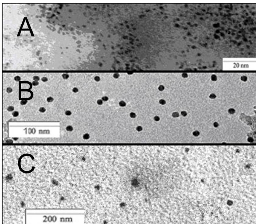
Figure 7: TEM image of Pt nanosized particles modified by cinchonidine (A), cinchonidine on Fe (B), quiphos on Pt (C). [R. Richards and A. Kraynov]
