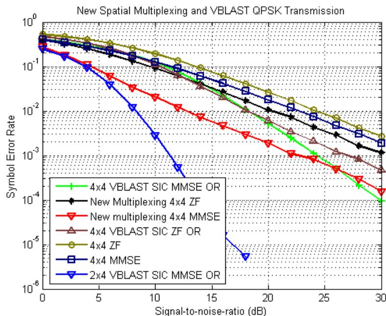
Figure 4: The bit-error performance of a new data multiplexing technique for multiple antenna transmission is compared against state-of-the-art solutions. (H. Haas et al.)
