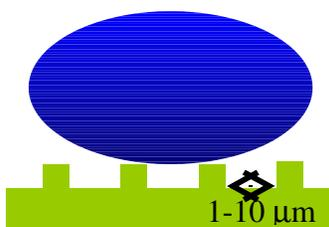
Figure 8: The Lotus effect, schematic. (F. Müller-Plathe)
