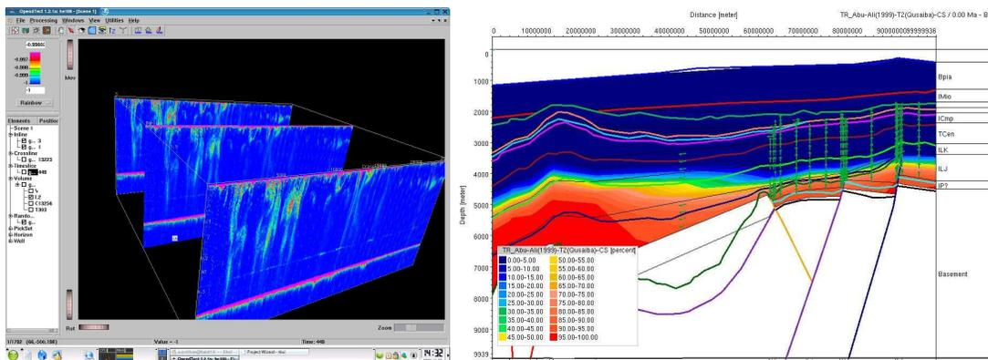
Figure 16: Left: Visualisation of parametric echosounder data showing of seafloor gas seepage in the North Sea. Right: Depth profile showing results from Petroleum System's Modelling of the Norwegian Margin. Green arrows indicate the direction of hydrocarbon migration while the colours represent hydrocarbon generation maturity. (V. Unnithan et al.)
